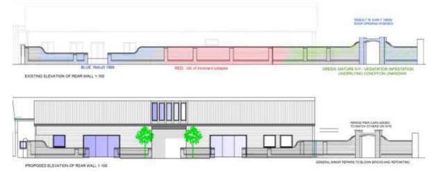
Figure 2 Works to the wall at the rear of the studio building
